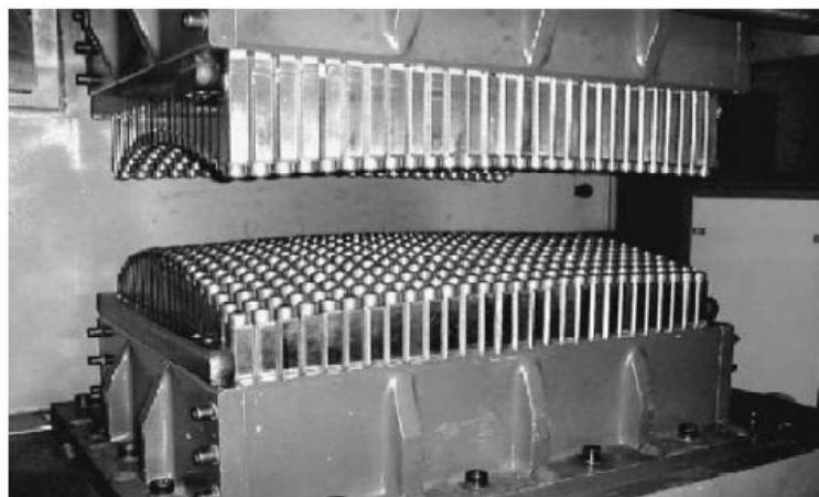
Figure 1.2: Tool for multi-point forming (Li et al., 2002).
