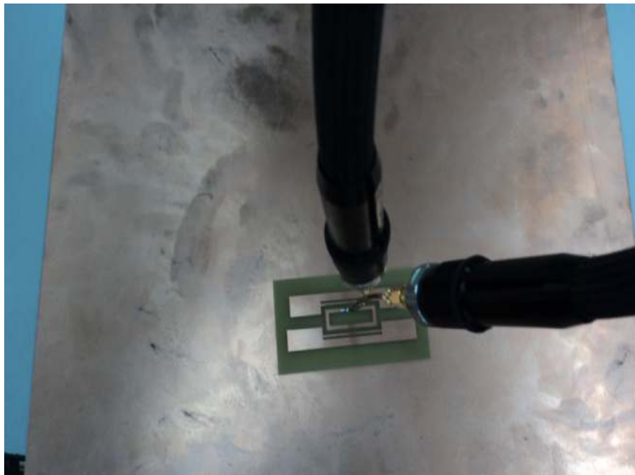
Figure 5.4: Measuring of the antenna input impedance when mounting on metal plate
