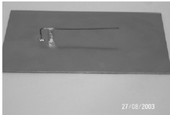
Figure 2.10: A fabricated IFA antenna (Ukkonen et al., 2004)
