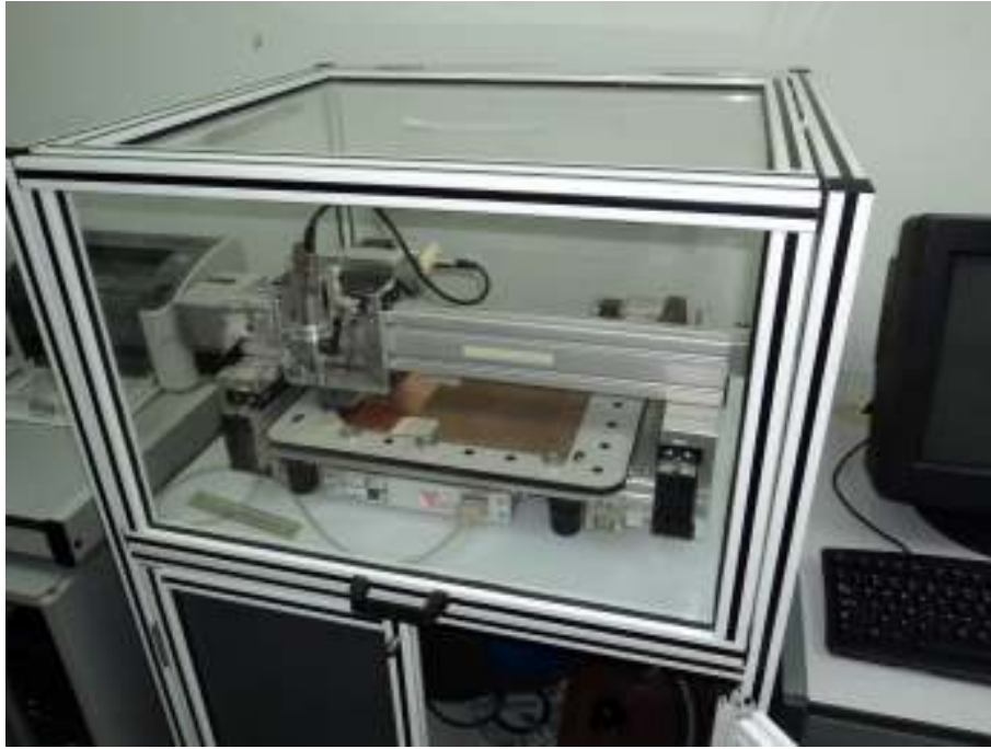
Figure 4.2: Cutting process of the FR-4 substrate using CNC milling machine
