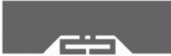
Figure 2.24: Microstrip patch antenna with T-matching network (M. Eunni, 2007)
