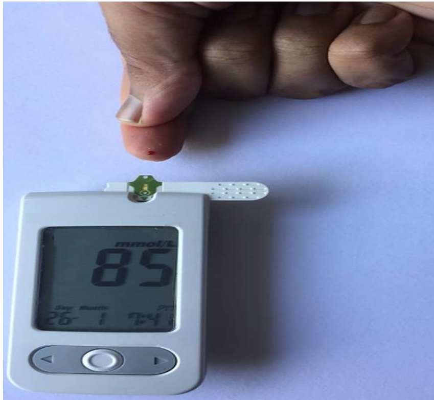
Figure 1.1 Commercially available –semi-invasive glucose biosensor or commonly known as the glucose meter.
