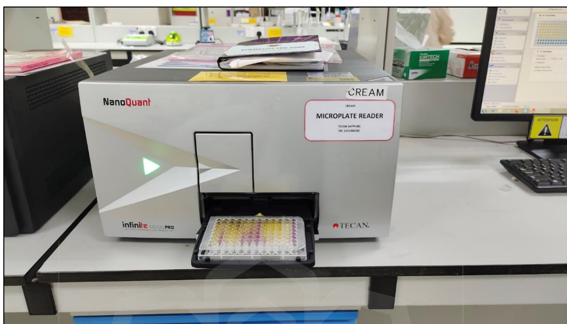
Figure 3.8 TECAN microplate reader used to measure absorbance
