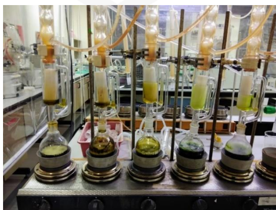
Figure 3.3 Soxhlet apparatus setup for the extraction of S. alata leaves.
