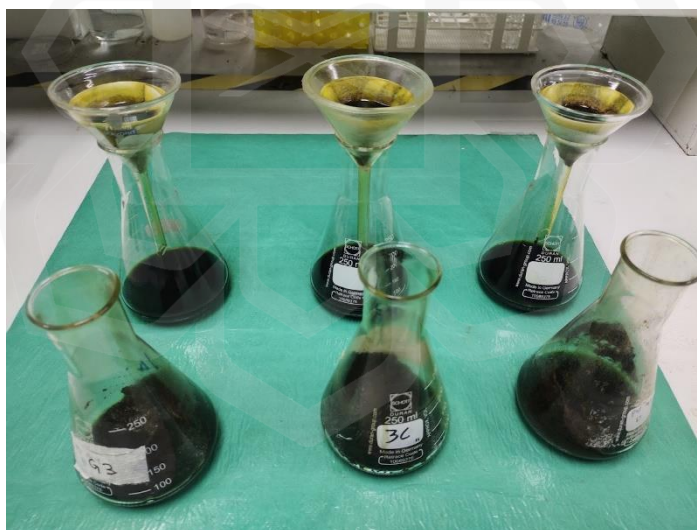
Figure 3.4 Filtration process for the separation of solid particles from the macerated extracts.
