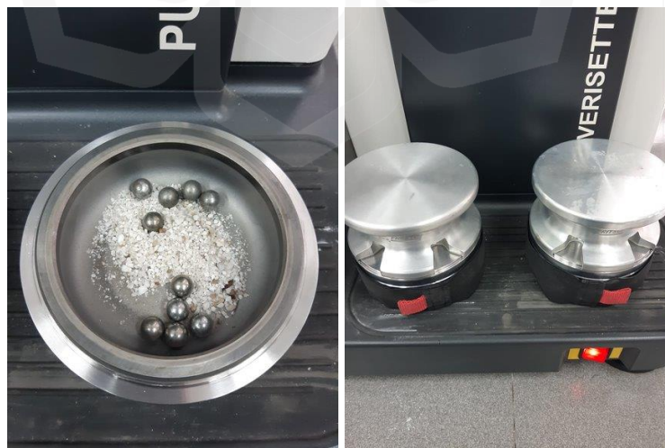
Figure 3.3: Raw sand placed inside jar with balls (left), jar enclosed tightly (right)
