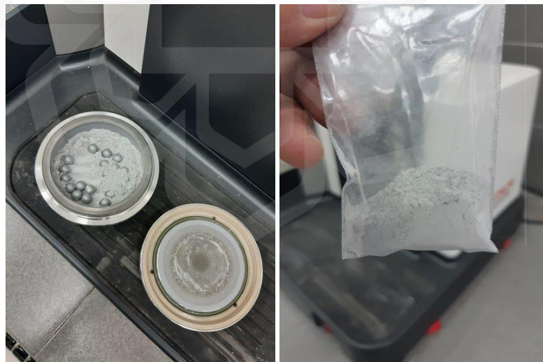
Figure 3.5: Crushed silica sand product (left), samples taken in small plastic bag for further characterization process(right)
