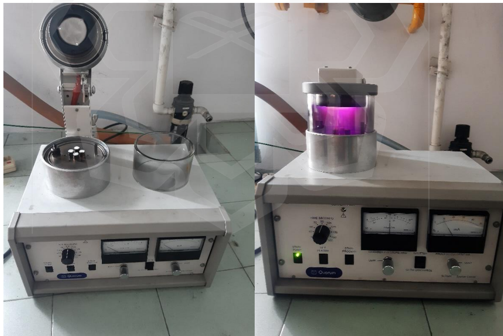
Figure 3.8: Silica sample inside chamber (left), coating process of silica sand (right)
