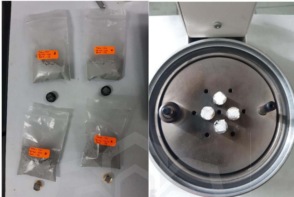
Figure 3.7: Silica sample placed on capsule (left), sample placed inside coating chamber
