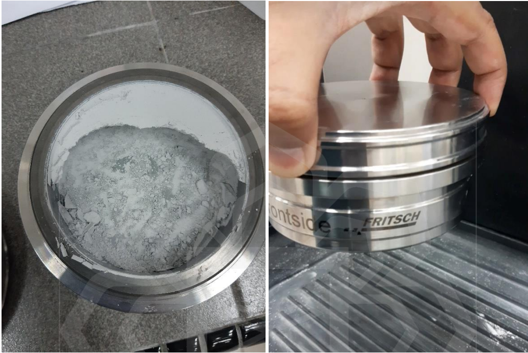
Figure 4.5: Silica sand turns to solid at 200 RPM (left), and jar enclosure can hardly be opened at 300 RPM (right)
