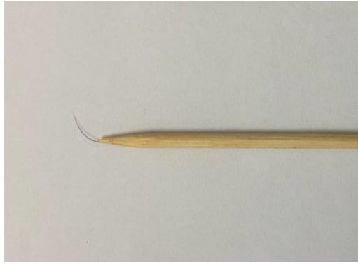
Figure 3.3 The eyelash pick Stub with carbon tape.
