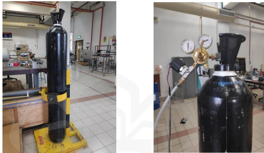
Figure 3.8 Oxygen tank (left), pressure gauge and regulator (right)
