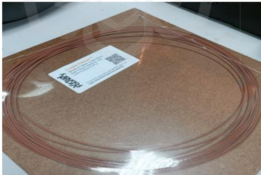
Figure 3.2 Sample of Copper Polymer Composite Filament used for the experiment
