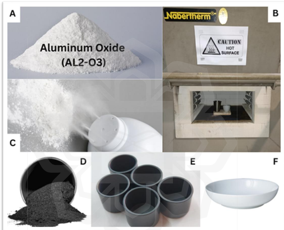
Figure 3.9 Images of the apparatus used in post processing: (A) Aluminum Oxide ( Al_2O_3 ), (B) Debinding and Sintering Furnace (C) Talcum Powder for Sintering (D) Sintering Carbon (E) Ceramic Crucible (F) Porcelain lid for crucible to conserve the sintering carbon
