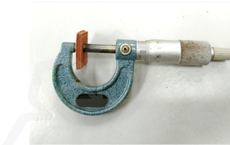
Figure 3.12 The above image shows the micrometer for measuring the values in z-axis
