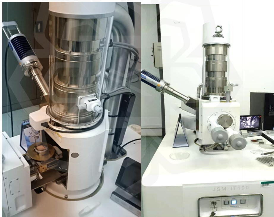
Figure 3.16 The above images show the Scanning Electron Microscope used for analyzing the microstructure of the samples
