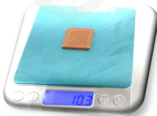
Figure 3.14 A mini electronic precision scale used for measuring the weight of the samples in grams
