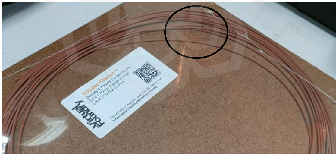
Figure 4.1 Illustrates the damaged part of the copper composite filament
