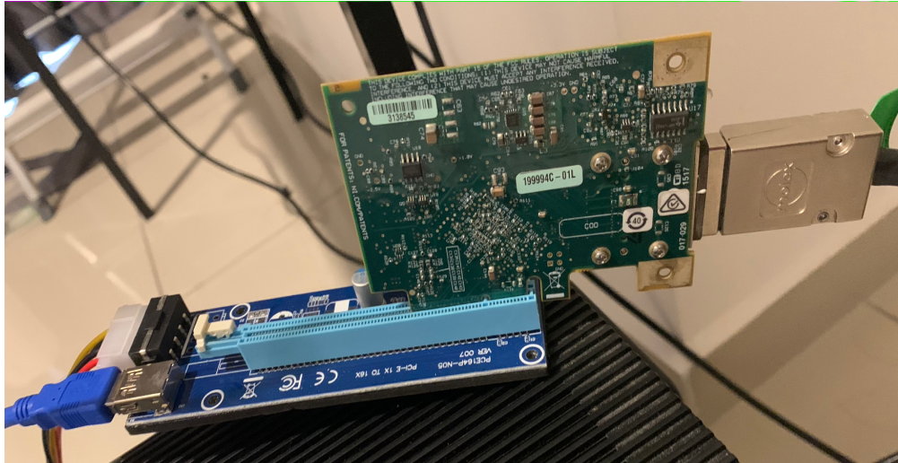
Figure 3.20 PCIe Extender and PCIe – MXI Express (PCIe 8371)
