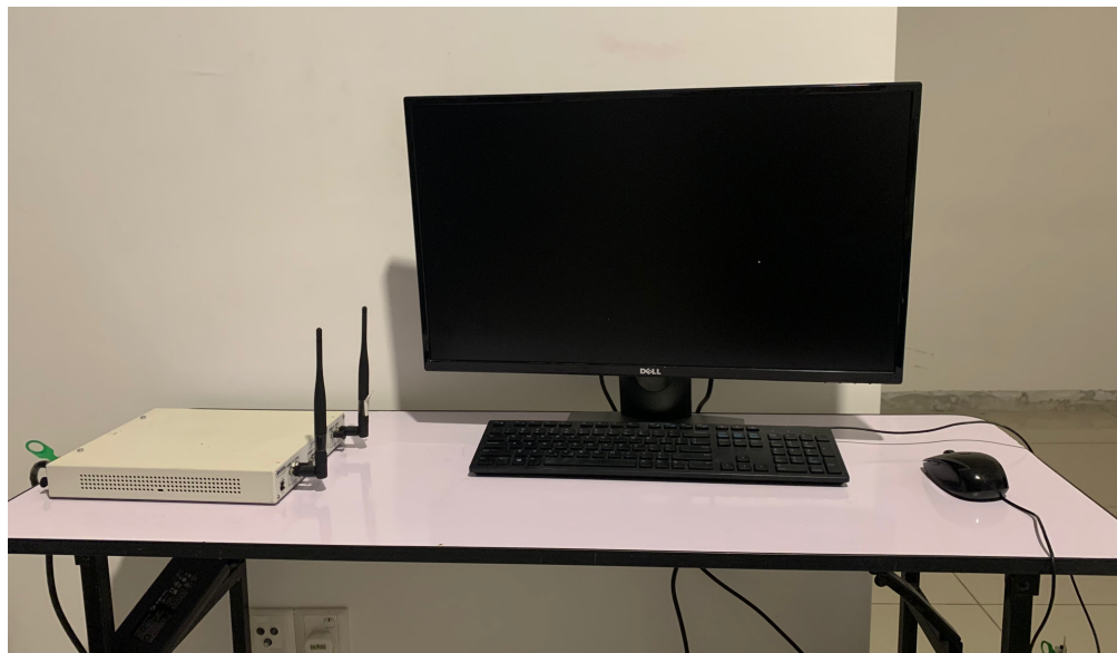
Figure 3.18 PC with LV Comm Software and NI USRP 2943R Transceiver
