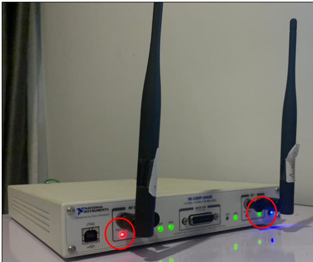
Figure 4.11 LED Lights for the Transmitter and Receiver for both OFDM and FBMC Configurations
