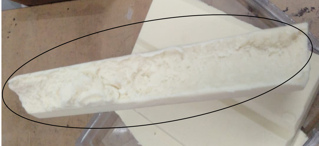
Figure 4.6 Porous type defect on white couverture chocolate.
