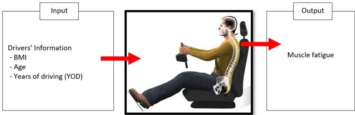
Figure 23 Block diagram of the mathematical model
