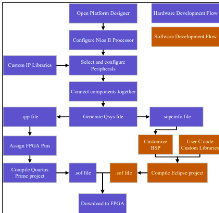
Figure 3.30 The Entire FPGA Development Flow
