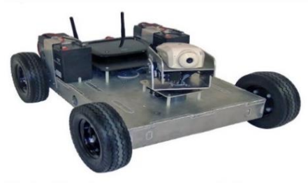
Figure 2.2: 4 Wheeled Non-Holonomic Robot
